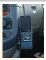
years. This hand held unit is compliant with Electronic Service Logs (E-Logs) that are used for Hours of Service (HOS) tracking and Electronic Driver Vehicle Inspection Reports (EDVIR) meeting the new regulations that will be implemented in the near future. We are in the process of rolling out of the hand held units and plan to be complete across all terminals by the end of 2014.
